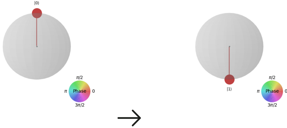
Figure 2.3: Transformation of |0\rangle to |1\rangle using the Y-gate
